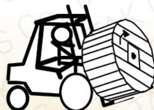
Drums may be lifted either by crane or fork-lift truck
