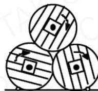
Only drums with protection lagging may be piled flange on flange. Lower layer to be secured over full drum width.
