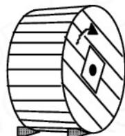
Keep the drum standing upright, using wedges in the heels of the flanges
