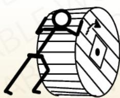
Roll the drum in the direction used during cable reeling
